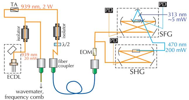
Fig. 1. Schematic diagram of the laser setup.
