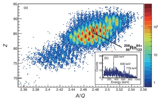
Fig. 1. (a) Particle identification plot for the RI beam measured at the second stage of BigRIPS. The atomic number  $Z$  versus the mass to charge ratio is shown. (b) The  $\gamma$ -ray energy spectrum of the known isomeric state in  $^{208}\text{Rn}$ , indicated by the circle in (a). Three  $\gamma$ -ray peaks can be clearly observed.
