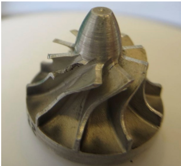
Fig. 4. T1 expansion turbine wheel with broken blades.
