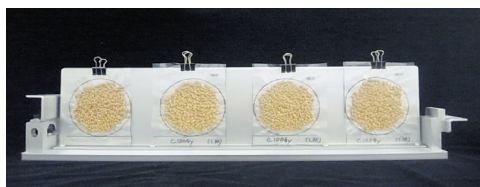
Fig.1 Rice seeds set into a cassette of automatic sample changer in our irradiation system. 5) Each bag contains three hundreds seeds of Nipponbare.
